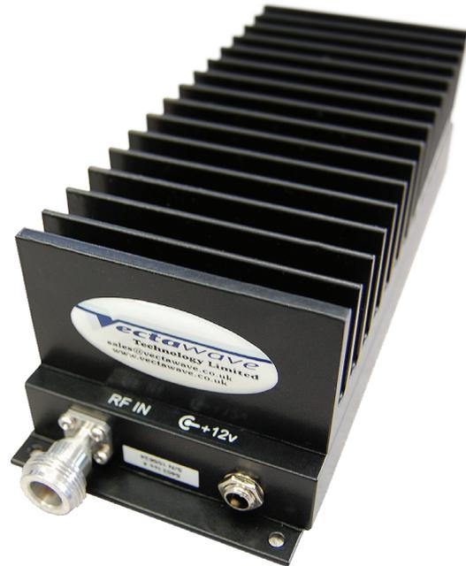
Model **VBM2500-3** is a solid-state amplifier capable of generating 3W minimum power over the 10-2500MHz frequency range. The amplifier is designed to operate from a 12V DC supply, and so is applicable for either equipment bus or battery operation.
