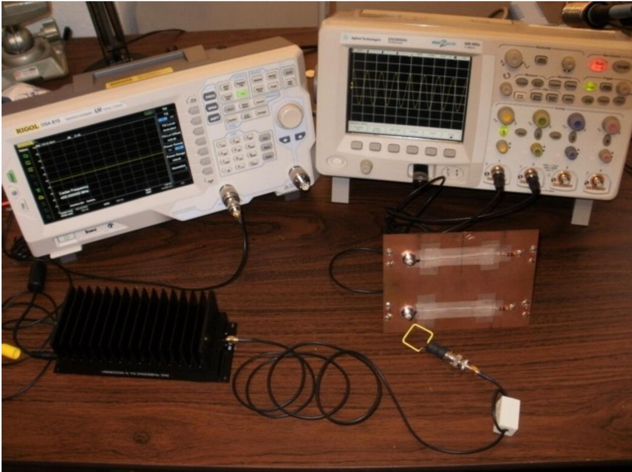
**Figure 2.** Test Setup to Investigate RF Induction into a PCB with a Ground Plane Break
