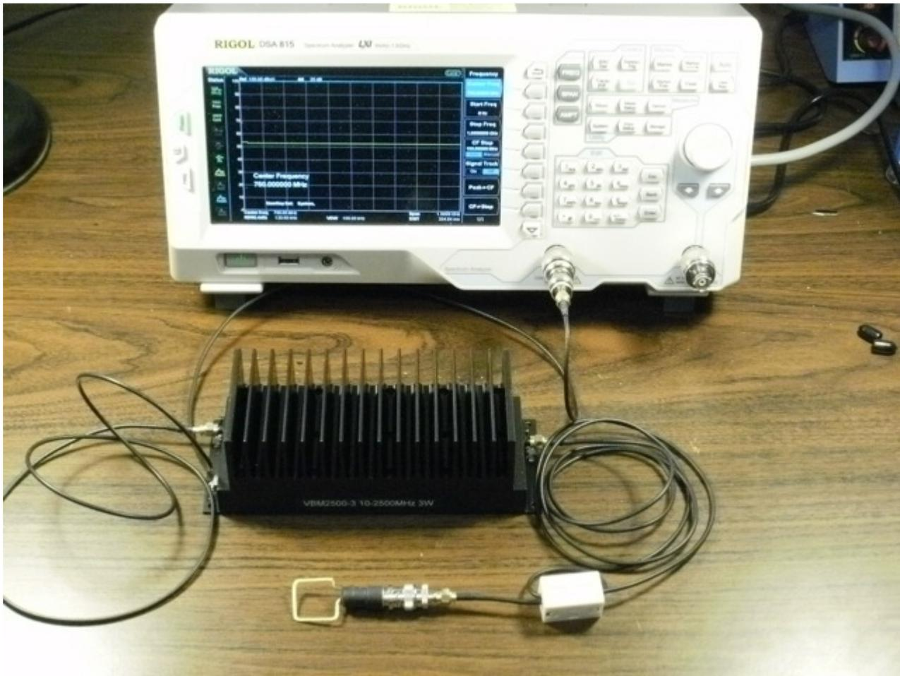
**Figure 1.** Test Setup for Troubleshooting Radiated and Conducted Immunity Problems
