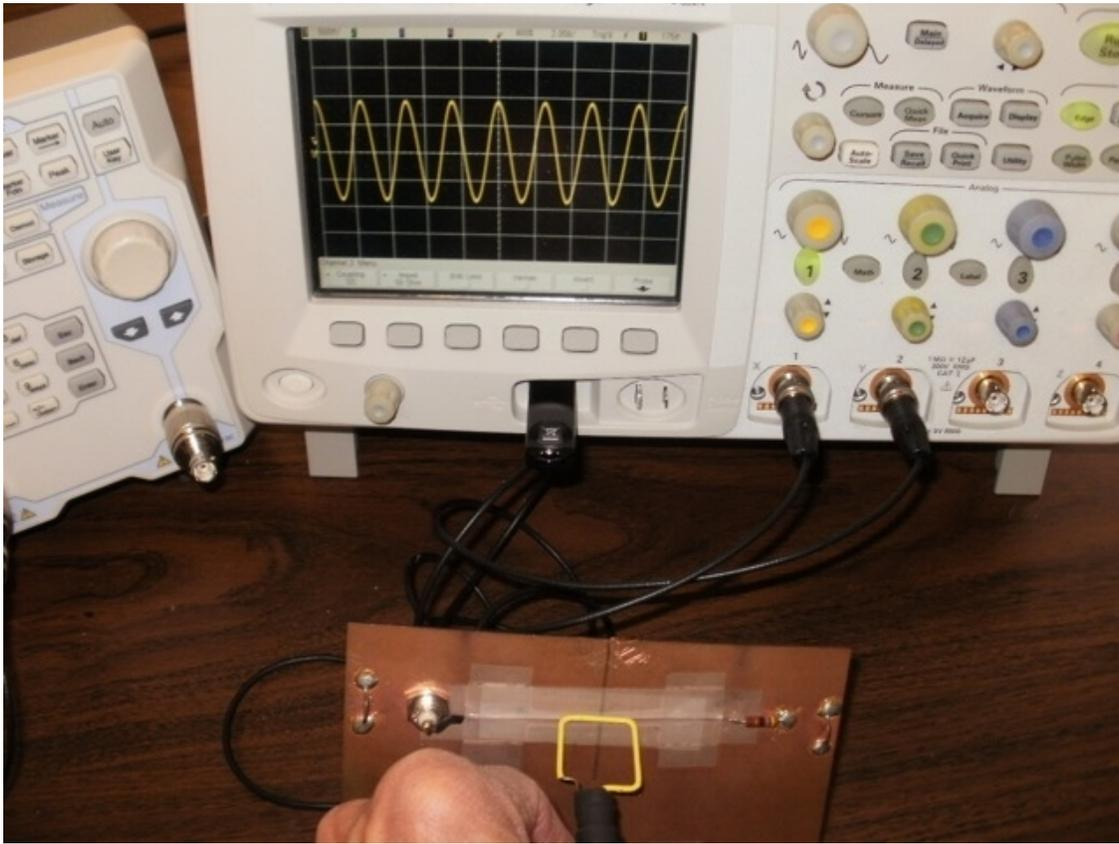
**Figure 3.** RF Signal Injection Into Path on the Test Board
